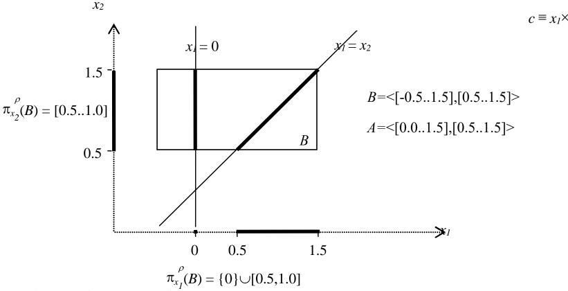
*B* is not box-consistent  $(0 \notin [-0.5, -0.499] \times ([0.5, 1.5], -[-0.5, -0.499]) = [-1, -0.498])$  *A* is box-consistent:
