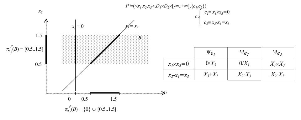
The inverse interval expressions are associated with the primitive constraints of the decomposed CCSP P'
